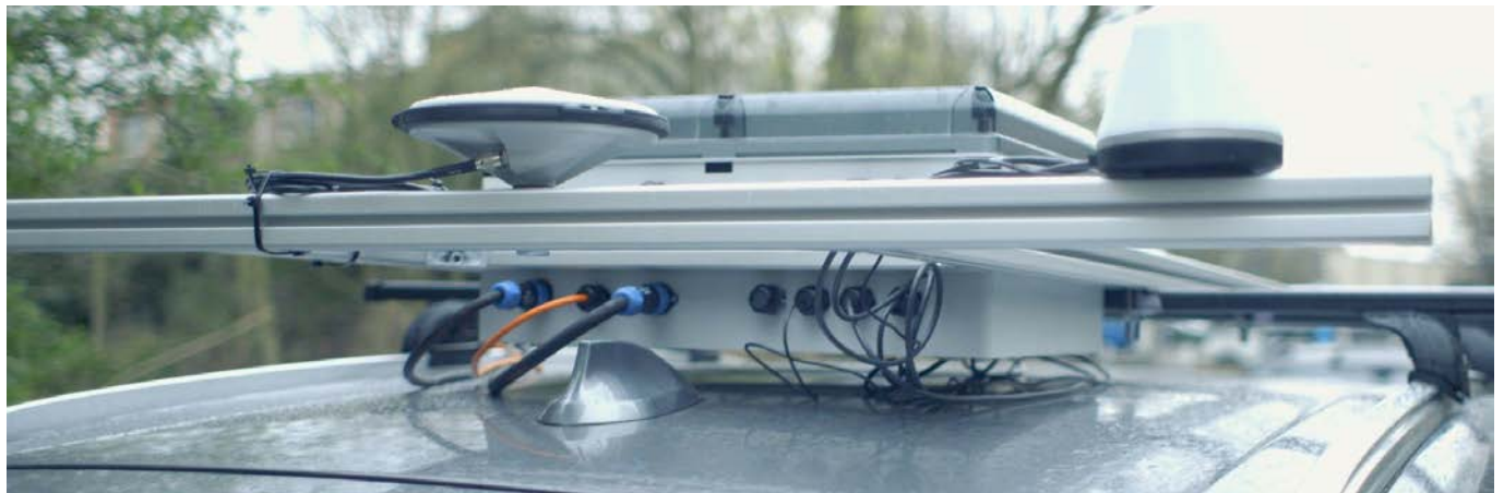
Imec’s car-mounted communication units support 4G LTE, Direct C-V2X and ITS-G5 / DSRC (and allow to flexibly switch between these technologies) for thorough and objective testing. Source: imec
