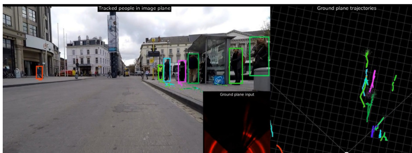
Field tests in the City of Ghent (Belgium), 2019 – featuring cooperative (radar and video) sensor fusion. Source: imec.
